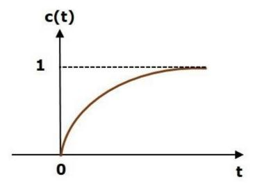
The value of the **unit step response**,  $\mathbf{c}(\mathbf{t})$  is zero at t=0 and for all negative values of t. It is gradually increasing from zero value and finally reaches to one in steady state. So, the steady state value depends on the magnitude of the input.
