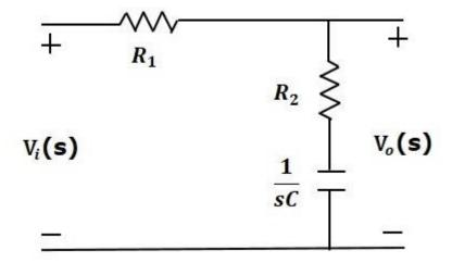
Here, the capacitor is in series with the resistor  $R^2R^2$  and the output is measured across this combination.
