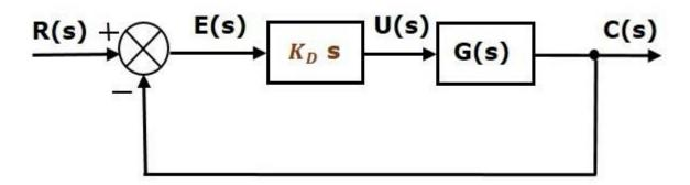
The derivative controller is used to make the unstable control system into a stable one.
