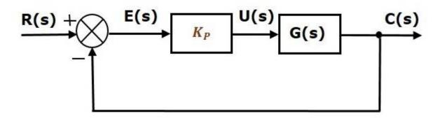
The proportional controller is used to change the transient response as per the requirement.
