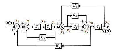
Represent the input signal R(s) and output signal C(s) of block diagram as input node R(s) and output node C(s) of signal flow graph.
