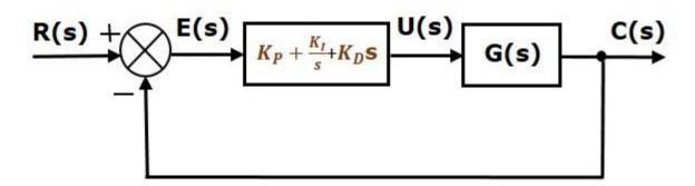
The proportional integral derivative controller is used to improve the stability of the control system and to decrease steady state error.
