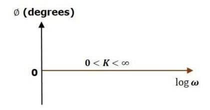
The magnitude plot is a horizontal line, which is independent of frequency. The 0 dB line itself is the magnitude plot when the value of K is one. For the positive values of K, the horizontal line will shift  $20\log K_{20\log K} dB$  above the 0 dB line. For the negative values of K, the horizontal line will shift  $20\log K_{20\log K} dB$  below the 0 dB line. The Zero degrees line itself is the phase plot for all the positive values of K.
