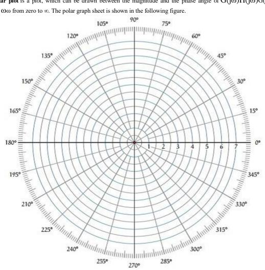
This graph sheet consists of concentric circles and radial lines. The concentric circles and the radial lines represent the magnitudes and phase angles respectively. These angles are represented by positive values in anti-clock wise direction. Similarly, we can represent angles with negative values in clockwise direction. For example, the angle 2700 in anti-clock wise direction is equal to the angle  $-90^{\circ}$  in clockwise direction.
