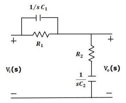
This circuit looks like both the compensators are cascaded. So, the transfer function of this circuit will be the product of transfer functions of the lead and the lag compensators.
