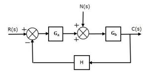
The **closed loop transfer function** due to noise signal alone is
