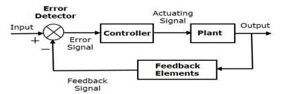
The error detector produces an error signal, which is the difference between the input and the feedback signal. This feedback signal is obtained from the block (feedback elements) by considering the output of the overall system as an input to this block. Instead of the direct input, the error signal is applied as an input to a controller.
