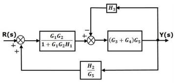
**Step 4** – Use Rule 3 for blocks  $(G_3+G_4)G_5$  and  $H_3$ . The modified block diagram is shown in the following figure.
