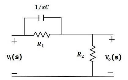
Here, the capacitor is parallel to the resistor R<sub>1</sub>R<sub>1</sub> and the output is measured across resistor \$R 2.
