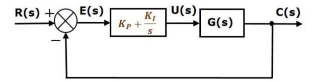
The proportional integral controller is used to decrease the steady state error without affecting the stability of the control system.
