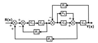
**Step 1** – Use Rule 1 for blocks  $G_1$  and  $G_2$ . Use Rule 2 for blocks  $G_3$  and  $G_4$ . The modified block diagram is shown in the following figure.
