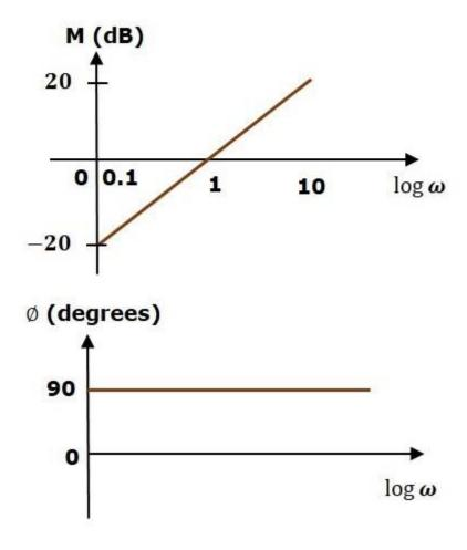
The magnitude plot is a line, which is having a slope of 20 dB/dec. This line started at  $\omega$ =0.1 $\omega$ =0.1 rad/sec having a magnitude of -20 dB and it continues on the same slope. It is touching 0 dB line at  $\omega$ =1 $\omega$ =1 rad/sec. In this case, the phase plot is 90 $^{0}$  line.
