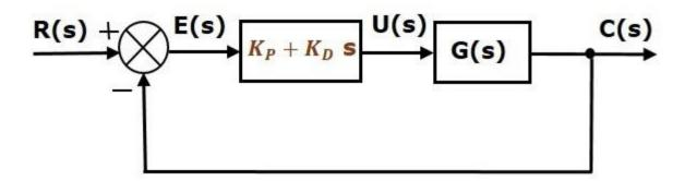
The proportional derivative controller is used to improve the stability of control system without affecting the steady state error.
