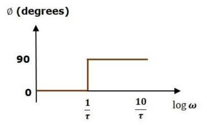
The magnitude plot is having magnitude of 0 dB upto  $\omega=1\tau\omega=1\tau$  rad/sec. From  $\omega=1\tau\omega=1\tau$  rad/sec, it is having a slope of 20 dB/dec. In this case, the phase plot is having phase angle of 0 degrees up to  $\omega=1\tau\omega=1\tau$  rad/sec and from here, it is having phase angle of 90°. This Bode plot is called the **asymptotic Bode plot**.
