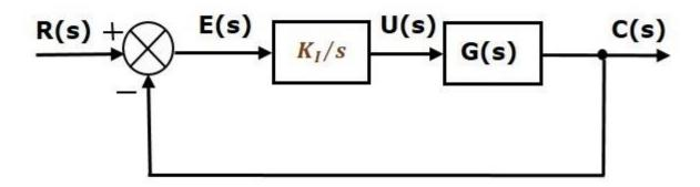
The integral controller is used to decrease the steady state error.
