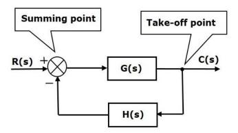
The above block diagram consists of two blocks having transfer functions G(s) and H(s). It is also having one summing point and one take-off point. Arrows indicate the direction of the flow of signals. Let us now discuss these elements one by one.
