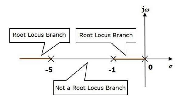
The three poles are located are shown in the above figure. The line segment between s=-1s=-1 and s=0s=0 is one branch of root locus on real axis. And the other branch of the root locus on the real axis is the line segment to the left of s=-5s=-5.
