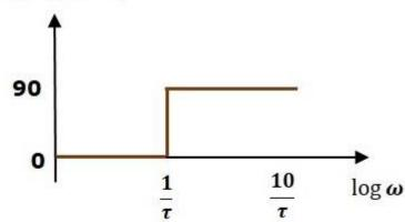
The magnitude plot is having magnitude of 0 dB upto  $\omega=1\tau\omega=1\tau$  rad/sec. From  $\omega=1\tau\omega=1\tau$  rad/sec, it is having a slope of 20 dB/dec. In this case, the phase plot is having phase angle of 0 degrees up to  $\omega=1\tau\omega=1\tau$  rad/sec and from here, it is having phase angle of 90°. This Bode plot is called the **asymptotic Bode plot**.
